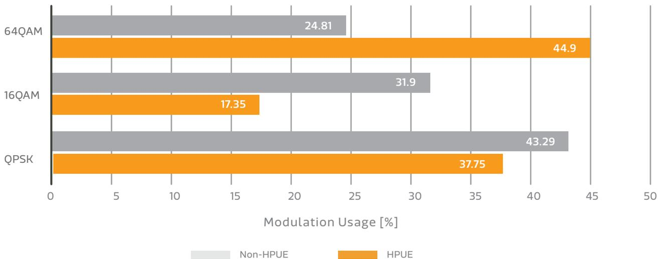
Figure 2 HPUE vs. non-HPUE Uplink Modulation Utilization in Mobility
