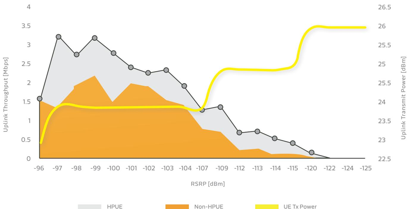
Figure 1- HPUE vs. non-HPUE Uplink Throughput Performance in Mobility
