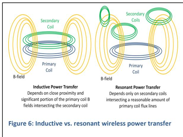
Figure 6: Inductive vs. resonant wireless power transfer
