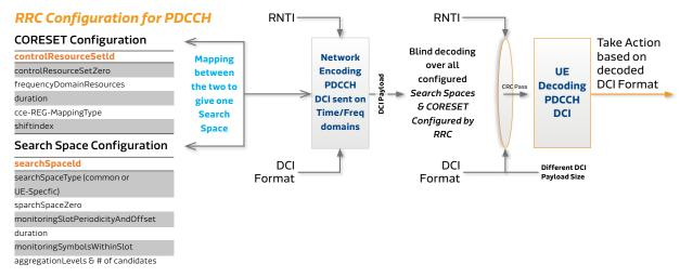
Figure 1 PDCCH DCI Blind Decoding.
