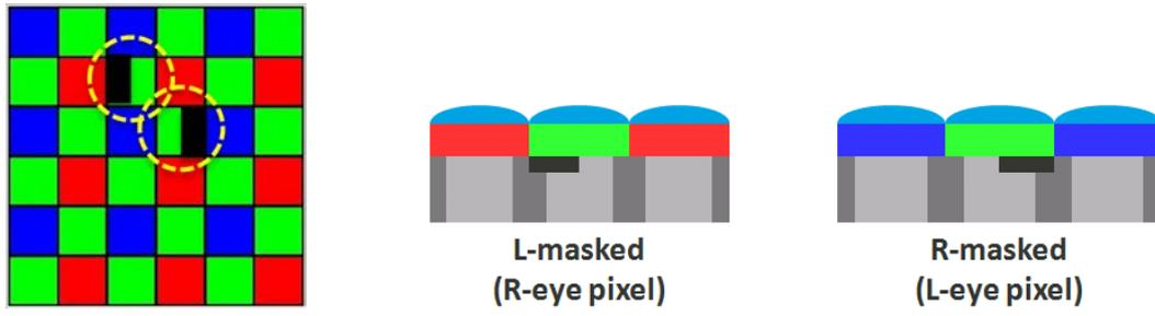
**Figure 5. PD Pixel Structure inside Image Sensor**
