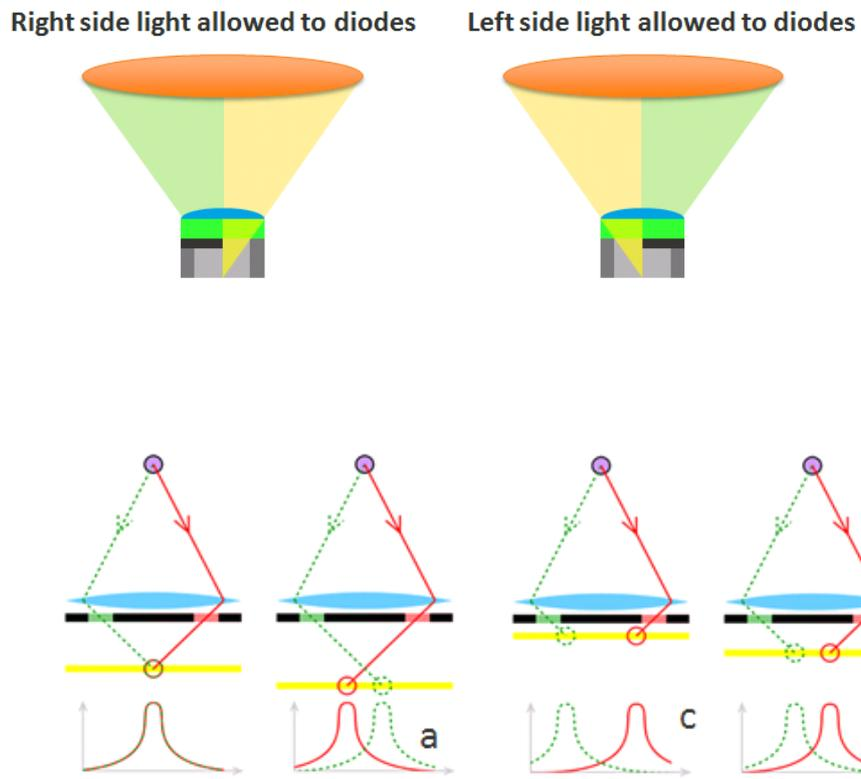
**Figure 6. Phase Difference from Two Signals**
