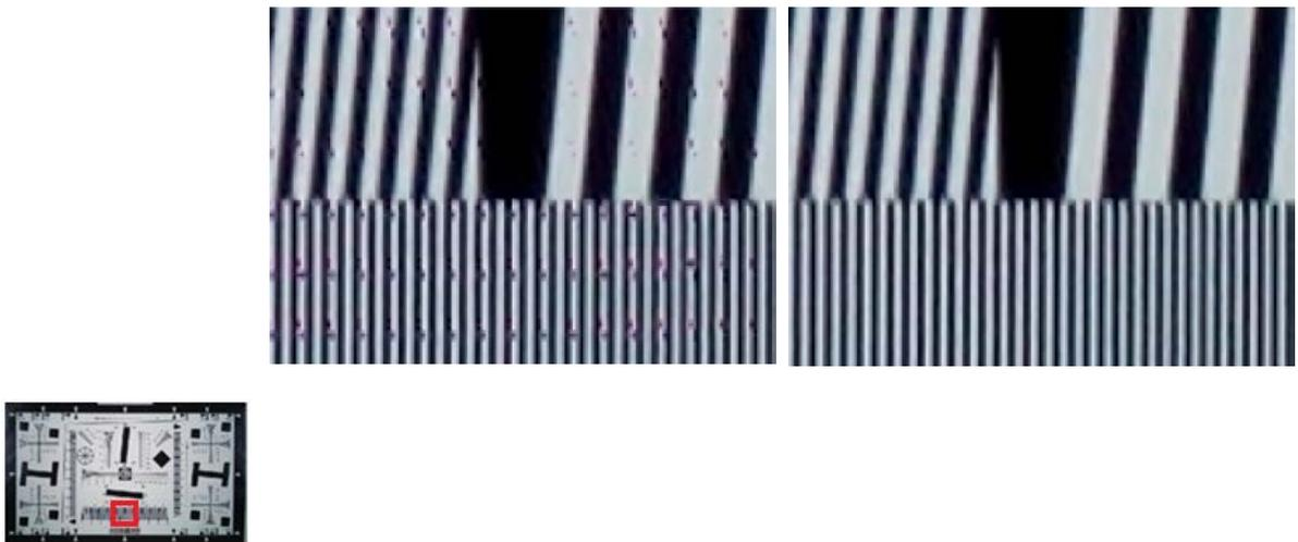
*Figure 4. PD Pixels Compensation Result with Mediatek Advanced ISP*
