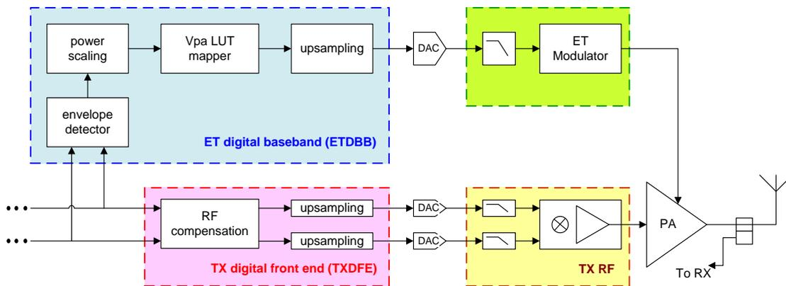
**Figure 3. MediaTek's Envelope Tracking System Block Diagram**
