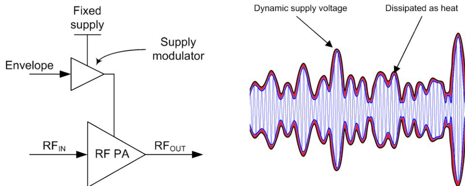
**Figure 2. Envelope Tracking Power Amplifier with Dynamic Supply Voltage**
