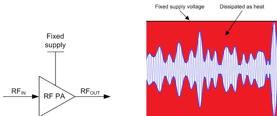
**Figure 1. Conventional Power Amplifier with Fixed Supply Voltage**
