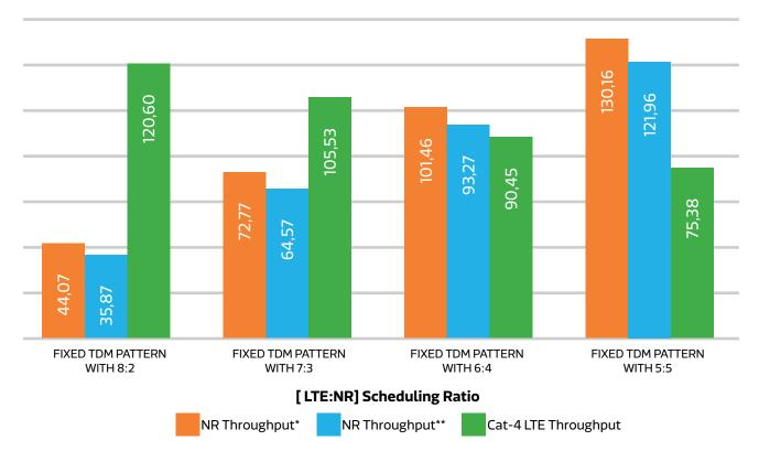
Figure 21. NR and LTE Downlink Throughput (Mbps) in DSS Operation with Different **TDM Patterns**
