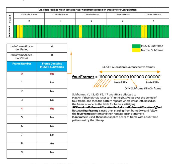
Figure 19. MBSFN Subframes Configuration for DSS Operation
