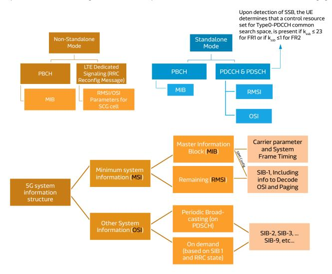
Figure 9. System Information in 5G NSA vs. SA Deployment
