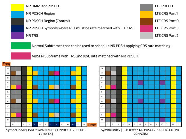
Figure 22. NR PDSCH Scheduling with LTE CRS Rate Matching in non-MBSFN subframes
