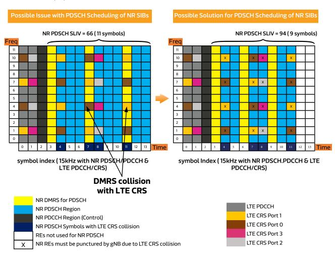
Figure 10. Impact of DSS on NR PDSCH and DMRS Resource Mapping in SA Deployment
