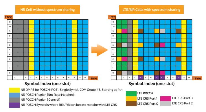
Figure 6. NR PDCCH/PDSCH SCS=15 kHz (without SSB)
