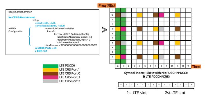
Figure 18. LTE Band & CRS Configurations inside NR Cell for DSS, configured to UE in rrcConnectionReconfiguration Message
