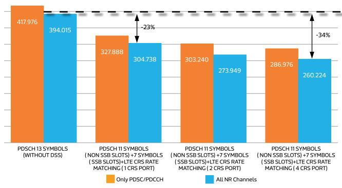
Figure 14. Maximum NR Slot Throughput (Mbps) for Case #4
