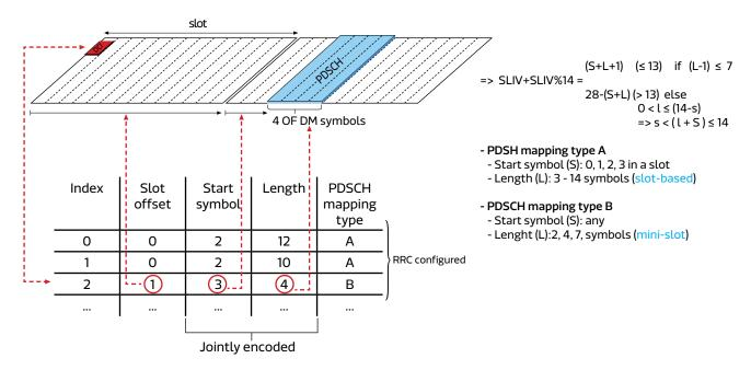
Figure 5. NR PDSCH Mapping Types in Time Domain
