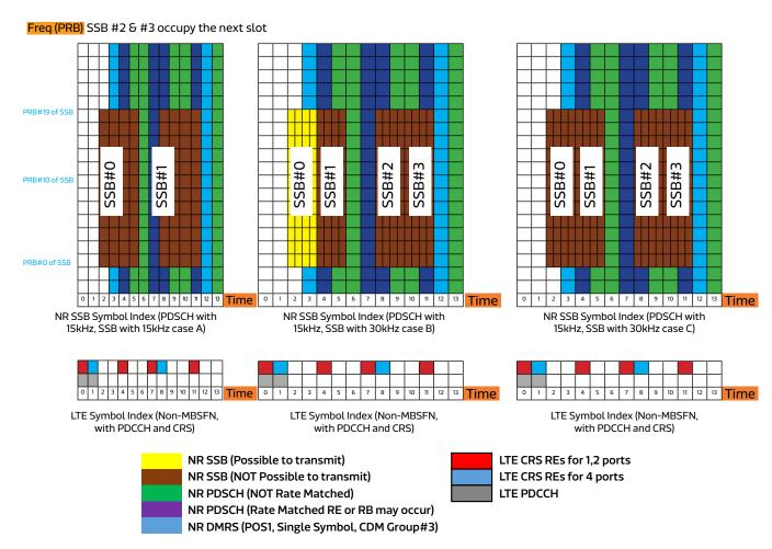
Figure 2. Impact of Spectrum Sharing on NR SSB Channel: Non-MBSFN
