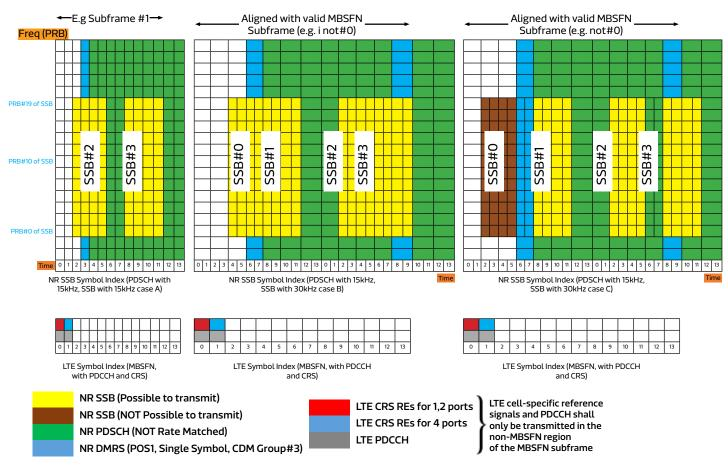
Figure 3. Impact of Spectrum Sharing on NR SSB Channel: MBSFN
