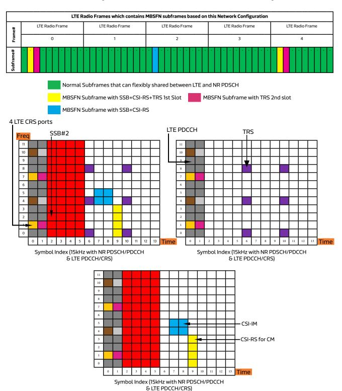
Figure 20. Overall View of NR and LTE Reference Signals in Time-Frequency
