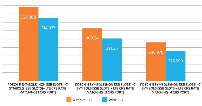
Figure 13. Maximum NR Slot Throughput (Mbps) for Case #3
