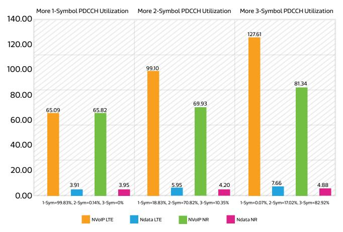
Figure 8. Average Number of Scheduled Users/Cell in b3/n3 with 20 MHz, SCS=15 kHz and 2x2 MIMO
