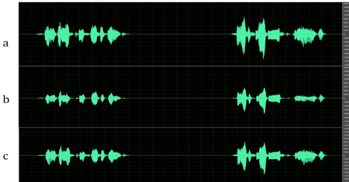
Figure 4. (a): Main microphone received signal, (b): Enhanced signal from general DMNR algorithm, (c): Enhanced signal from MEDIATEK's robust DMNR algorithm
