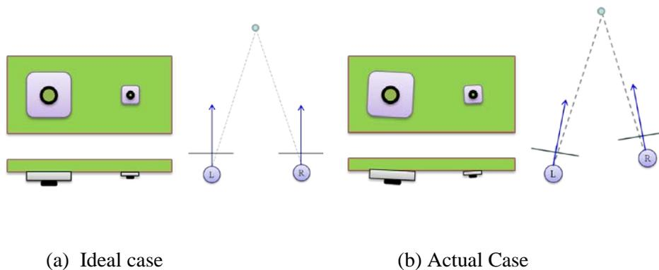
**Figure 4. Stereo Geometry of Asymmetric Dual Sensors**
